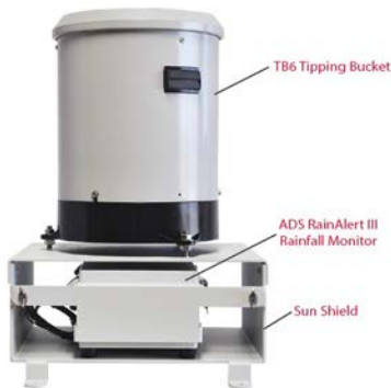
ADS RainAlert III Rain Gauge The ADS RainAlert III Rainfall Monitor with tipping bucket and sun shield, provides automated remote rainfall measurement and alarming.
