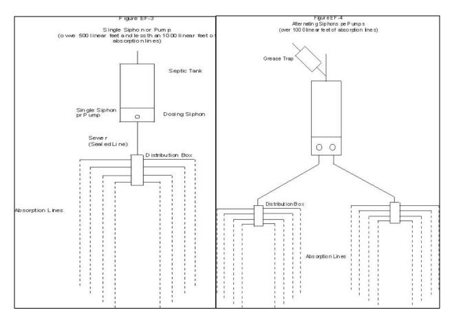
g. Design and Operation of Dosing Tank with Pump(s).
