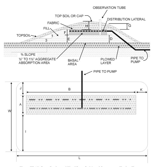
Figure FF-15 Cross Section and Plan View of a Mound System on a Sloping Site
