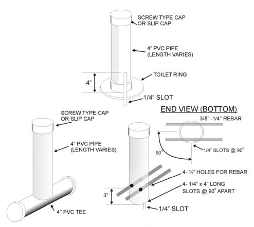
Figure FF-18 Three Methods for Stabilizing Observation Tubes
