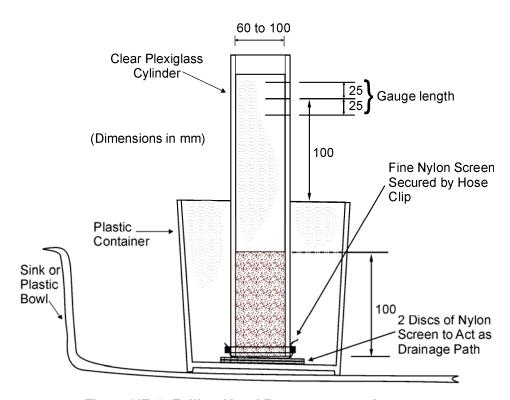
Figure HF-5 Falling Head Permeameter - Apparatus
