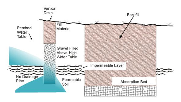
Figure HF-3 Underdrain Used to Lower Water Table
