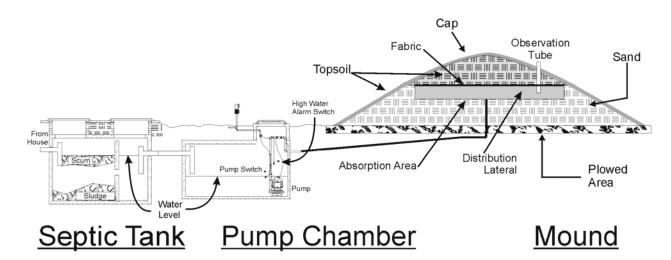
Figure FF-12 Across-setion of a septic tank-mound system for on-site disposal
