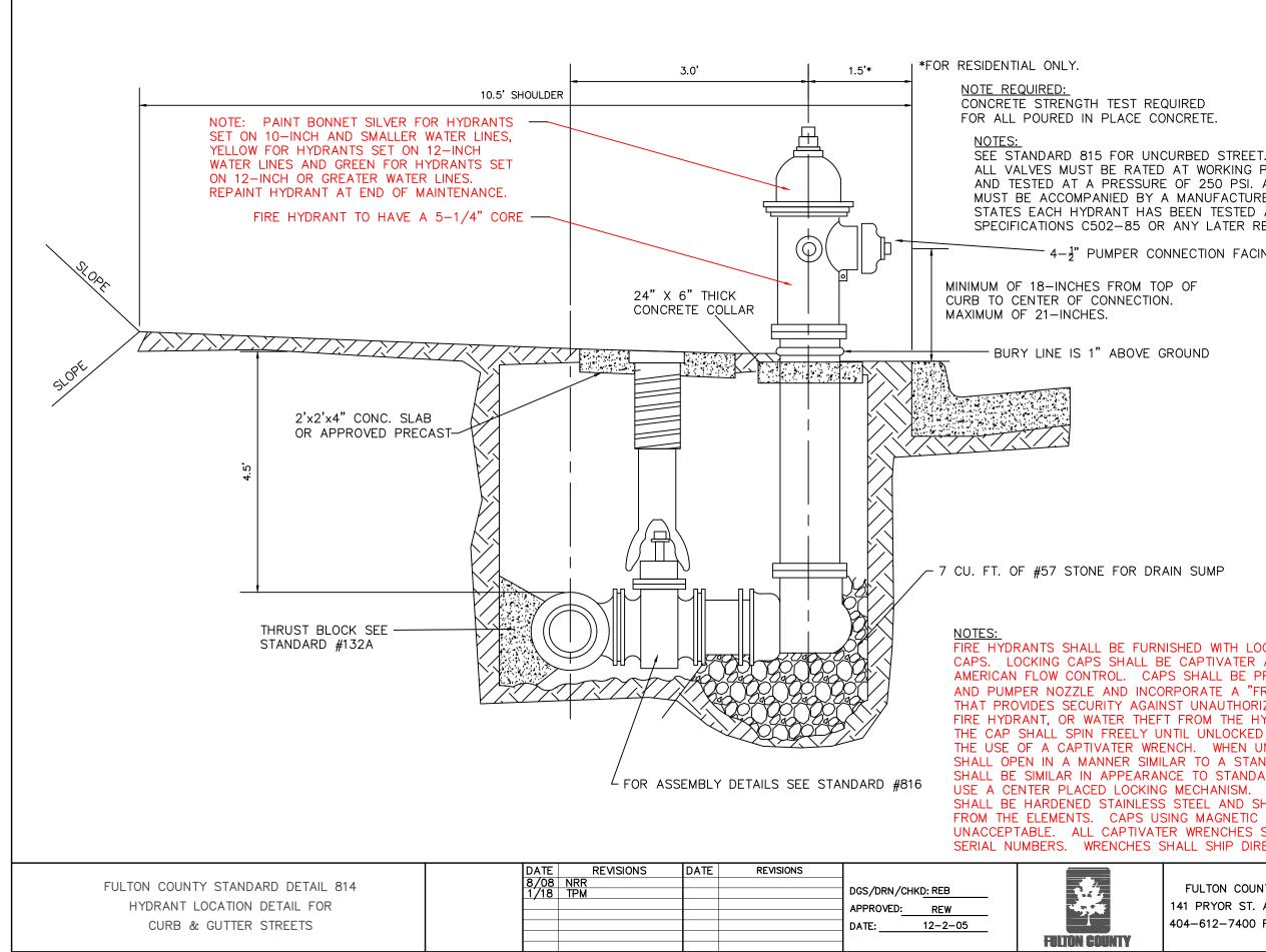
ALL VALVES MUST BE RATED AT WORKING PRESSURE OF 200 PSI AND TESTED AT A PRESSURE OF 250 PSI. ALL FIRE HYDRANTS MUST BE ACCOMPANIED BY A MANUFACTURERS CERTIFICATE THAT STATES EACH HYDRANT HAS BEEN TESTED AT AWWA SPECIFICATIONS C502-85 OR ANY LATER REVISION.
