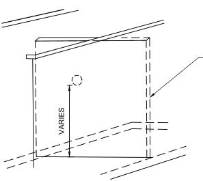
BAFFLE STANDS 50" IN HEIGHT AND IS  $2\frac{1}{2}$ " IN THICKNESS REINFORCED W/ 6-6-10 WIRE MESH
